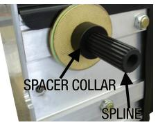
4. Install the Spline and the Spacer Collar.
